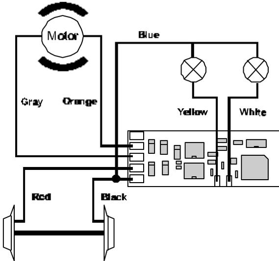
Figure 1: Wiring the LE103XF using track voltage common
