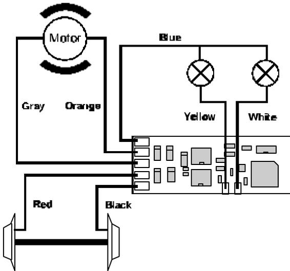
Figure 2: Wiring the LE103XF using a floating common.
