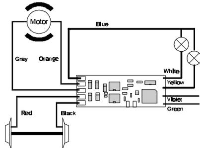
**Figure 2: Wiring the LE105XF using a floating common.**
