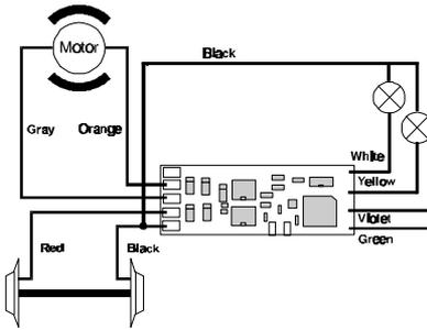
**Figure 1: Wiring the LE105XF using track voltage common**
