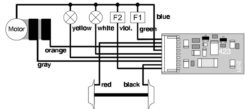
Figure 2: Wiring the LE122 using a track voltage floating common.
