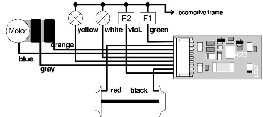
Figure 1: Wiring the LE122 using
