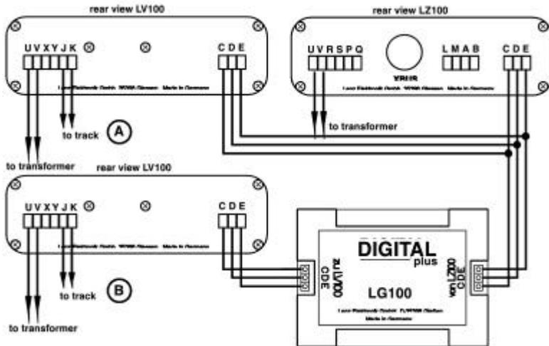
Illustration 1: Connecting the brake module to LZ100 and LV100
