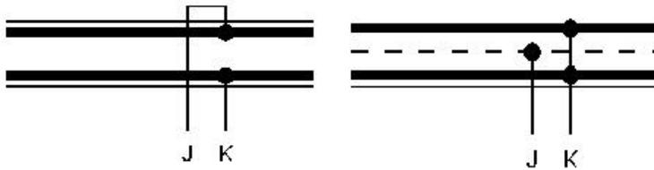
**Figure 2 Connecting 2-rail track** **Figure 3 Connecting 3-rail track**
