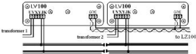
**Figure 4 Connecting track voltage when using 2 LV100**
