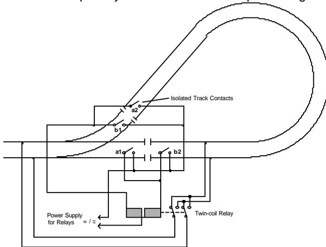
**Figure 6: Wiring of Reverse Loops**
