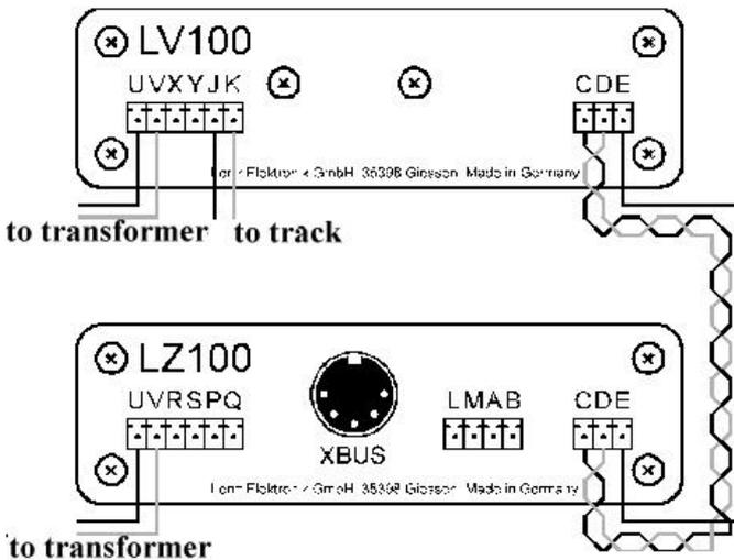
**Figure 1 Connecting LV100 to Command Station LZ100**
