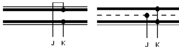
Figure 2 Connecting 2-rail track Figure 3 Connecting 3-rail track
