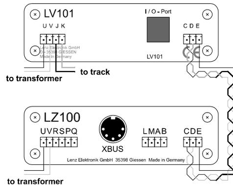
Figure 1 Connecting LV101 to Command Station LZ100
