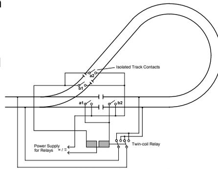
**Figure 5: Wiring of Reverse Loops**
