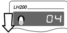
Set the direction switch so that the locomotive will operate in the proper direction when added to the consist. In this example #4 will operate in the reverse direction as the consist.
