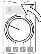
Turn the rotary control-knob back to the left. The locomotive slows down, the further you turn the knob to the left the more it will slow down (Throttle positions decrease in size).
