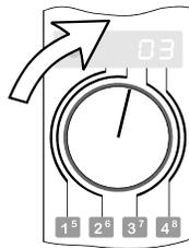
Turn the rotary control-knob to the right. The locomotive moves forward, and the more you turn the knob to the right, the faster the locomotive will move (Throttle positions increase in size).
