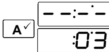
In the display the relevant digit address alternates with 4 horizontal bars. At this stage it is still possible to stop the deletion. To do so press the "0"key.
