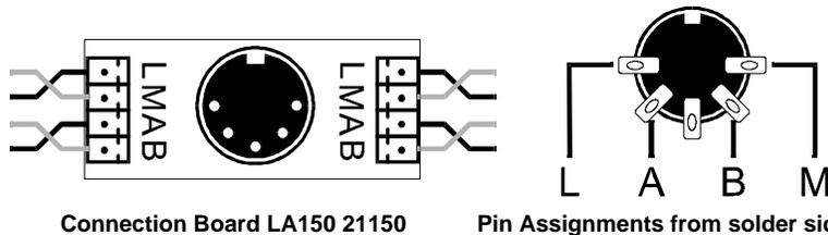
**Make sure that you do not mix up the cables of the terminals L and M. This could result in a short in the connected input devices.**
