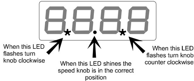
Now place the direction switch in the correct position, up (forwards) or down (backwards). If the upper dot appears in the middle of the display, then you must move the switch up (the forwards position). If the lower dot appears in the middle of the display you must move backwards switch it down (the backwards position backwards).
