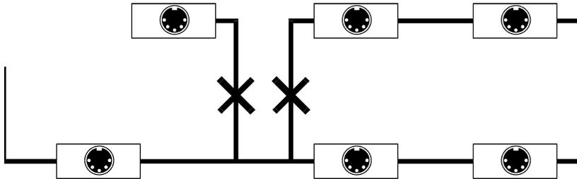
The ends of the XpressNET Network lines A and B should be connected to the resistor which is enclosed with the LA152 adapter. The resistor has a value of 120 Ohm.
